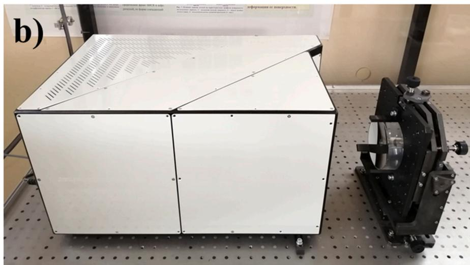
Fig. 2. (a) Diagram and (b) photograph of the interferometer in the process of measuring a spherical concave part.
